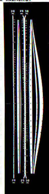
Fig. 7 Scales of the Metric RELASKOP in their full length. The varying width of the stripes illustrates how the instrument corrects for changes in slope. From left to right: tangent scale for horizontal distance of 20 meters, strip 1 with the following dark and two light bars, tangent scales for horizontal distances of 25 and 30 meters, strip 2, and two stripes of different width used as range finder.
